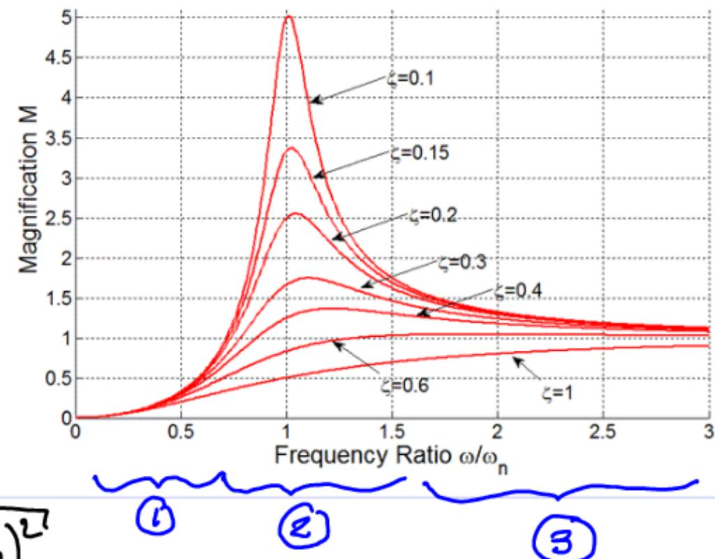
**5.6.11 Example:** A motor with total mass  $m + m_0 = 50\text{kg}$  has rotating internal mass of  $m_0 = 1\text{kg}$  that rotates on a shaft with eccentricity  $Y_0 = 1\text{mm}$  at angular rate  $\omega = 100\text{rad/s}$ . The engine is mounted on vibration isolation pads with effective stiffness  $k=500000\text{N/m}$  and a dashpot coefficient  $c=250\text{Ns/m}$ . The system is found to have a severe vibration problem. Which of the following changes will reduce the vibration amplitude?
