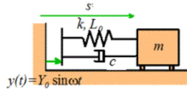
$$X_0 = KY_0 M(\omega, \omega_n, \zeta) \quad M = \frac{\left\{1 + (2\zeta\omega/\omega_n)^2\right\}^{1/2}}{\left\{(1 - \omega^2/\omega_n^2)^2 + (2\zeta\omega/\omega_n)^2\right\}^{1/2}} \quad \phi = \tan^{-1} \frac{-2\zeta\omega^3/\omega_n^3}{1 - (1 - 4\zeta^2)\omega^2/\omega_n^2}$$
