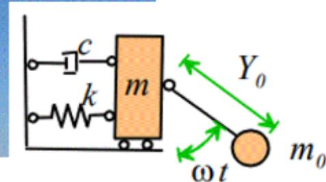
**5.6.12 Example:** An unbalanced wind turbine is idealized as a rotor excited spring-mass system. The mass  $m$  represents the tower, and  $m_0$  represents the combined mass of the three rotor blades. The rotor is 'unbalanced' because its center of mass is a distance  $Y_0$  away from the axle. The total mass of the turbine is 25000kg, the spring stiffness is 4100 kN/m and the dashpot coefficient is 128 kNs/m.
